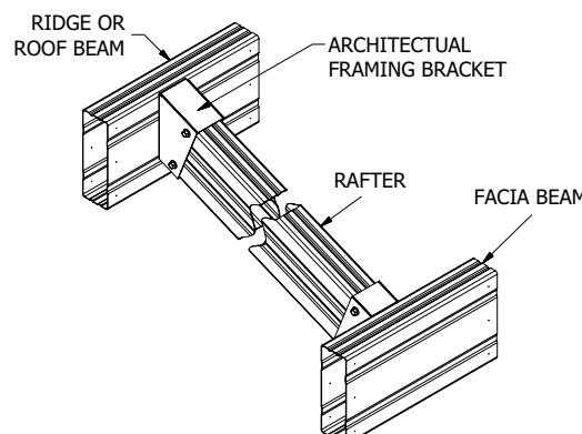
RAFTER TO ROOF BEAM CONNECTION
