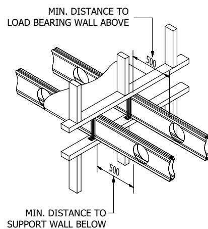
CUTTING SERVICE HOLES IN FLOOR JOISTS
