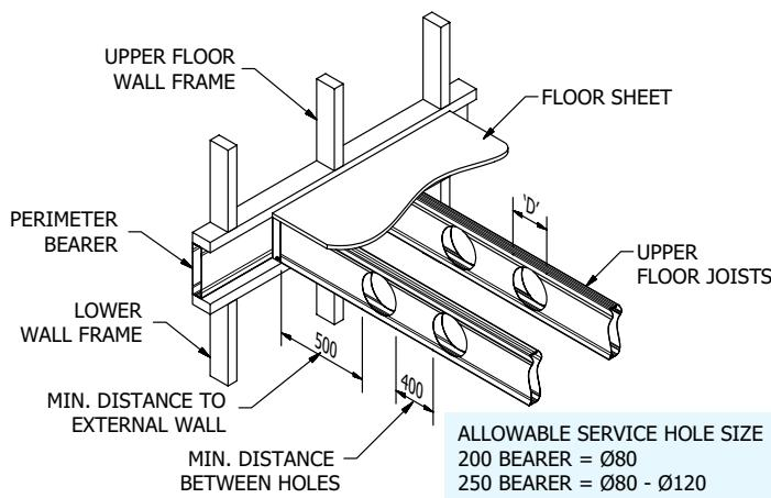
CUTTING SERVICE HOLES IN FLOOR JOISTS
